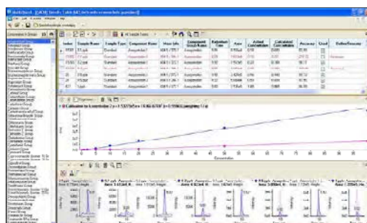
Figure 3. Azoxystrobin detected in a pesticide screening method using a QTRAP® 4500 system with highlighted outliers for the qualifier MRM transition at 0.1 and 0.2 ng/mL (calibration line of 0.1 to 100 ng/mL with r^2 = 0.999 and \%CV = 3.72\% at 1 ng/mL, n = 10 )
